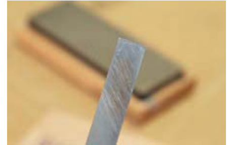
Starting to flatten back of chisel with diamond stone
