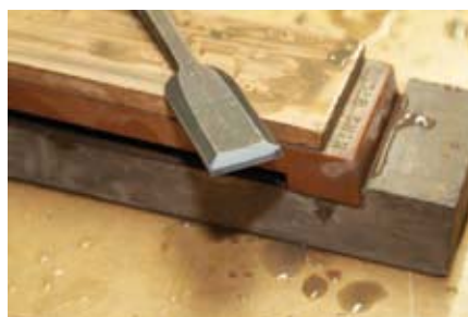
Honed and polished bevel on a Japanese chisel
