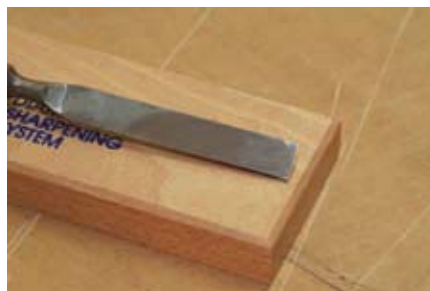
Back of chisel after flattening with diamond stone
