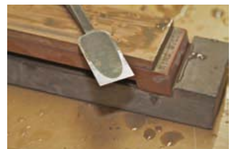
Mirror polished back of a Japanese chisel
