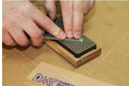
Flattening back with diamond stone
