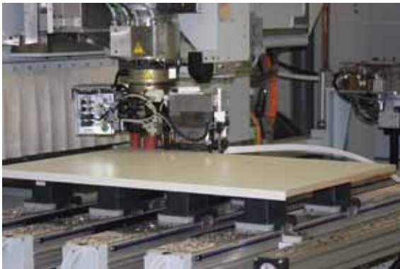
Left: The Homag processing center BAZ 322 with 5- axis spindle Drive5+ and edge banding unit.
