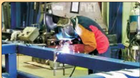
Welding of a heavy duty steel frame
