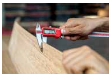
Thickcut veneers – checking the tolerances at Danzer.
