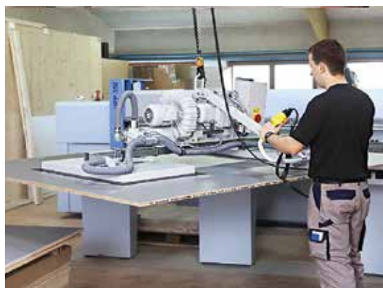
Far left: Vacuum lifting device VacuMaster Comfort for turning coated wooden boards by 180°.
