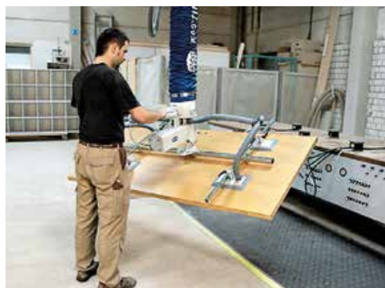
Far left: Vacuum tube lifter JumboErgo for loading and unloading a CNC machining centre.
