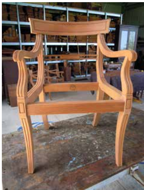
Cedar armchair c.1815. Before and after French polishing. From a set of four. Maker, Peter Gibbs.
