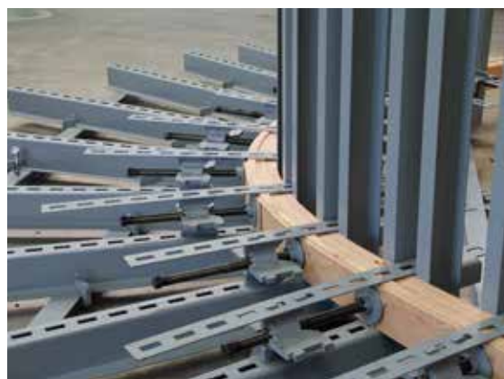
Curvwood's curved clamping system. Photo: Eva Dellow.
