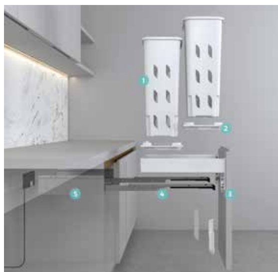
Concelo CRL235 laundry features (1) 35 litre hamper (2) Clip'n'Clean trays, (3) Door bracket with 6 way adjustment (4) 45kg soft close Matrix runners (5) Side mounting to suit System 32mm drilling.
