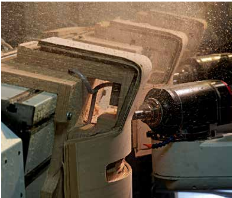
CNC contouring mills used for machining formed chair components. The components are clamped by vacuum
