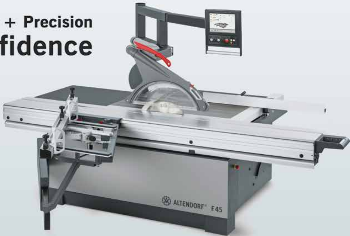
a Frictionless Surface. Sensitive veneer laminations or heavy panels are handled with ease on the Altendorf Air Cushion Table .
