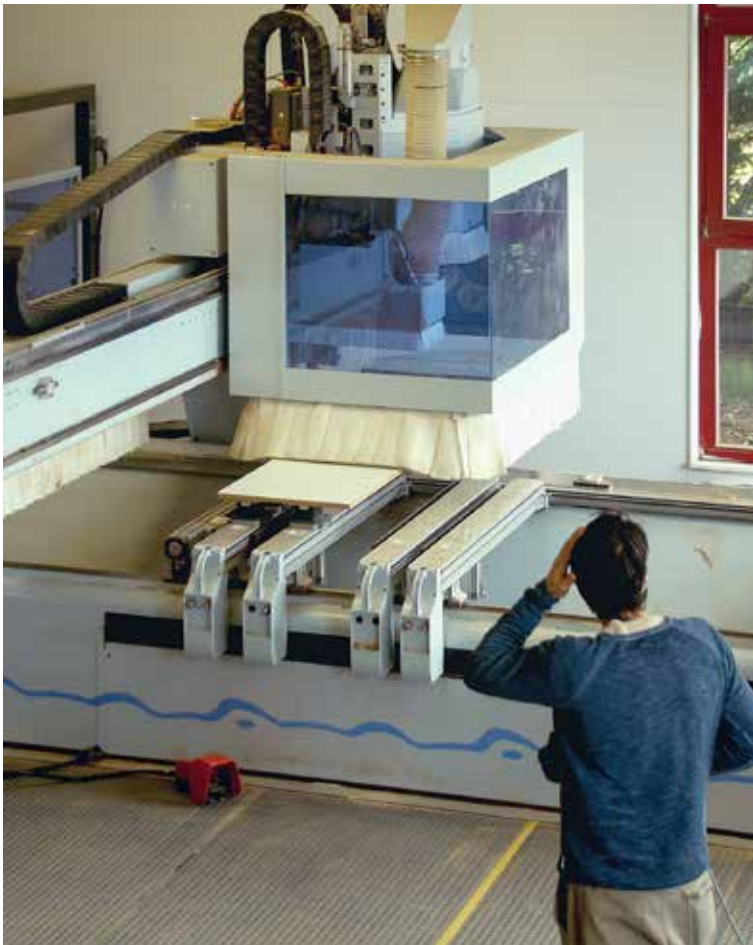
Benjamin Löw produces triangular boards with shift cuts on the 5 axis CNC machine
