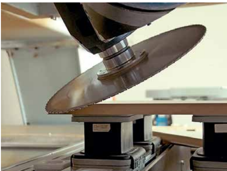
The NN saw blade from Leuco creates finish cuts ready for gluing
