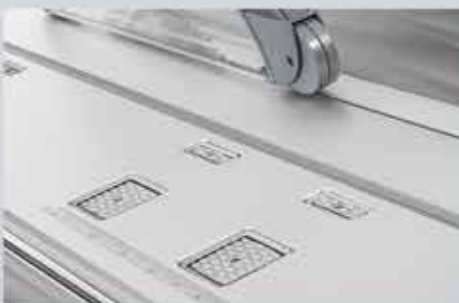
Vacuum Table. Secure and safe work piece hold down with various suction zones.
