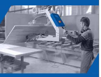
THE VACUMASTER 180° VACUUM LIFTER ALLOWS A HORIZONTAL LOAD TO BE LIFTED AND ROTATED 180° BY A SINGLE OPERATOR
