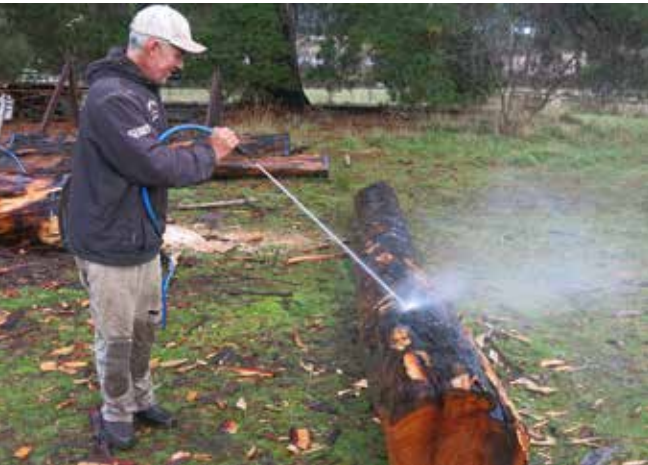
Left: Dave Golding washes off any remaining grit before the log faces the milling saw.
