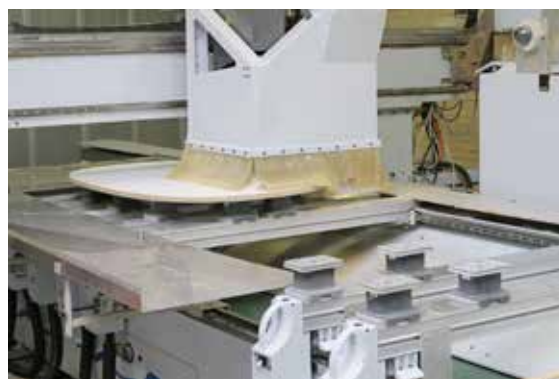
CNC router with consoles and vacuum blocks: while the work piece is being processed on one side, the finished work piece can be removed or reclamped on the other side.
