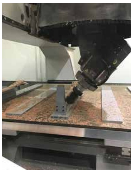
Machining guitar neck on Biesse Rover M5
