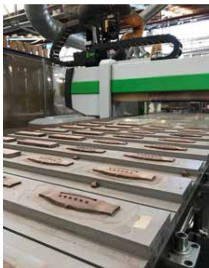
Completed guitar bridges on Biesse Rover C6
