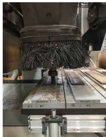
Machining ebony guitar fingerboard on Biesse Rover C6
