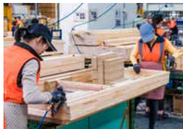
Compressed air is used here to power staple guns.
