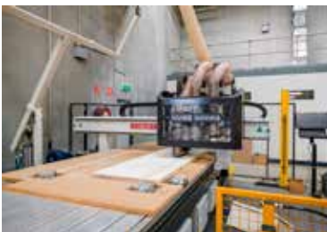
Compressed air is an important utility to Hume and can be found in use across the manufacturing process, here being used to power a CNC routing machine.
